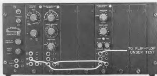
Figure 11. The basic Pulse Shaper arrangement.
