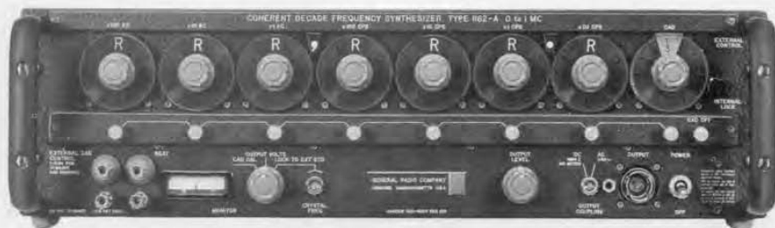
Figure 1. Panel view of the Type 1162-AR7C Coherent Decade Frequency Synthesizer with programmable decades. See complete listing of models on page 24.
